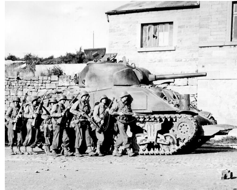
Combined arms in action: US M4 Sherman, equipped with a 75 mm main gun, with infantry walking alongside
