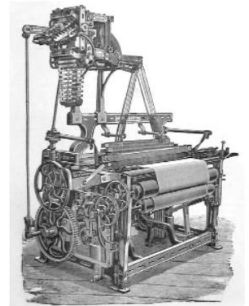
Sketch of a power loom (1892). image is courtesy of wikimedia commons and is public domain
