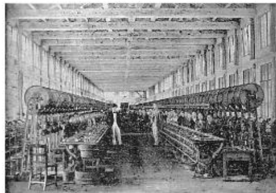
Photography of a Japanese silk factory in the early 1900s. The first factory of its kind was the Tomioka Silk Mill established in 1872 by the government to introduce modern machine silk reeling from France and spread its technology in Japan.
